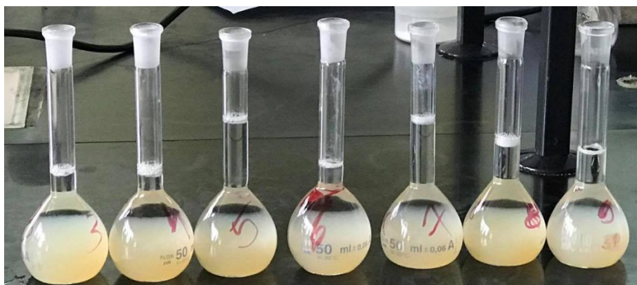
Figure 3 Samples ready for reading the absorbance on a spectrophotometer for HMF determination at two different wavelengths
